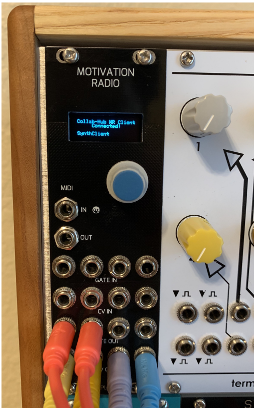
Figure 4: The Motivation Radio Eurorack module connected to the Collab-Hub server.
